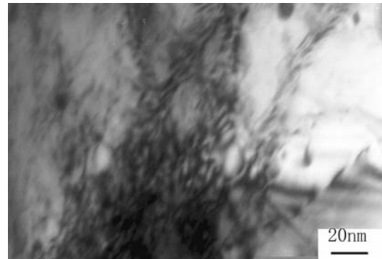
Fig. 10 Configuration of dislocations in the matrix adjacent to the graphite particulates
